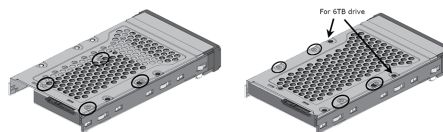
Figure 4, Secure the 2.5/3.5-inch Drive to the Tray
