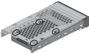
Figure 1-4-1. Installing 2.5-inch SAS/SATA Drive
