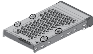
Figure 1-4-2. Installing 3.5-inch SAS/SATA Drive
